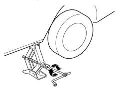
5. Remove the lug nuts by turning them counterclockwise; then remove the wheel.
